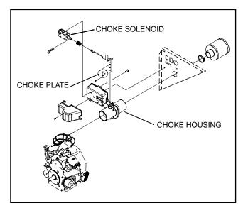
Figure 24. Exploded View Showing Location of Choke Plate - 10 kW Units
